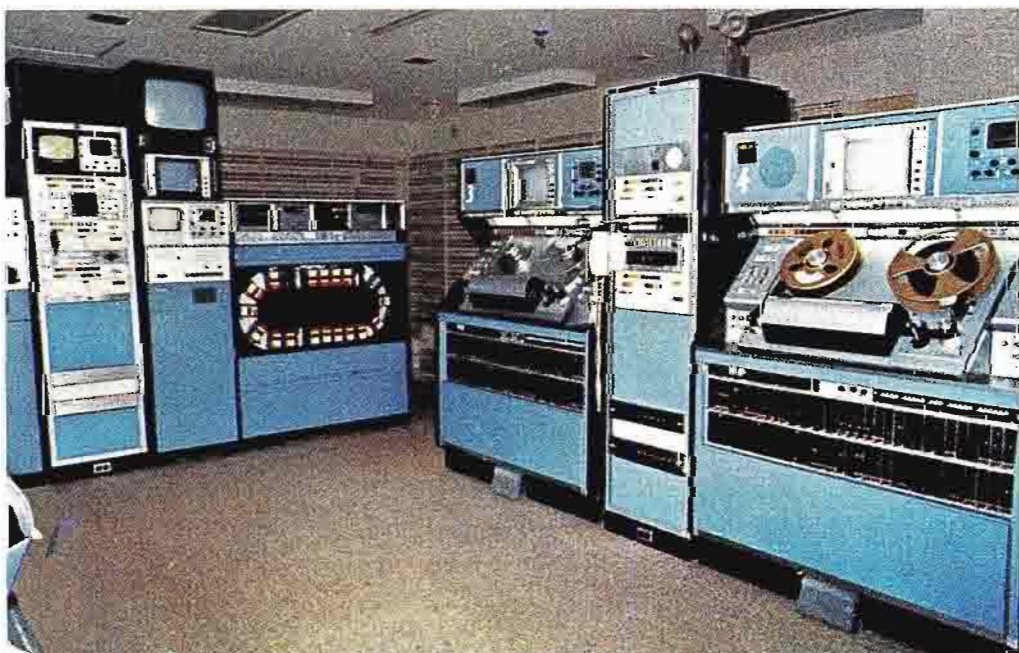
Two TCR-100A cartridge tape machines provide the flexibility needed for production and for on-air playback of "cart" commercials.
